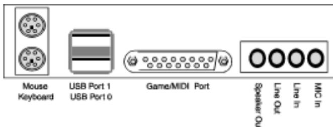
Figure 2.2: M55Hi-Plus Back Panel Connections
