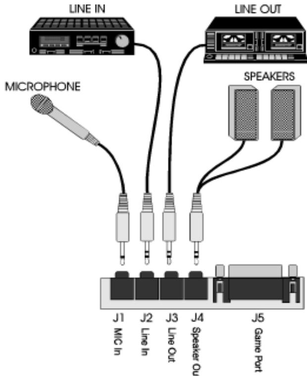
Figure 3-4: Connecting External Sound Devices
